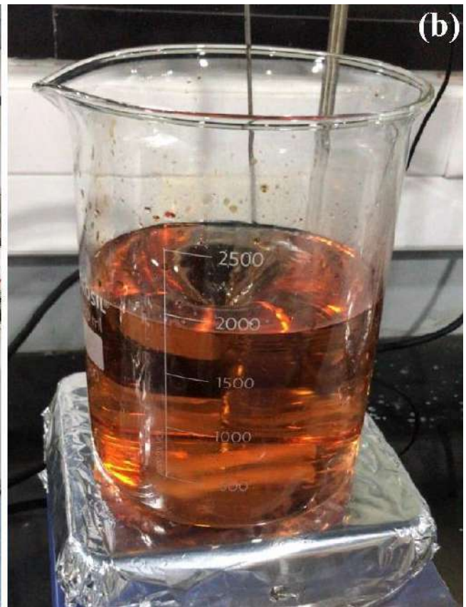
Fig.1: (a) 10L Autoclave facility and (b) sol-gel process for the scaled-up synthesis of Li-ion battery materials
