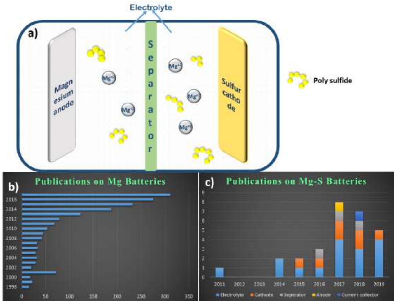
Figure 1. a) Schematic diagram of Mg-S battery working mechanism, b) Number of research articles published on Mg Batteries since 1998, c) Number of research articles published in Mg-S batteries (Till now).
