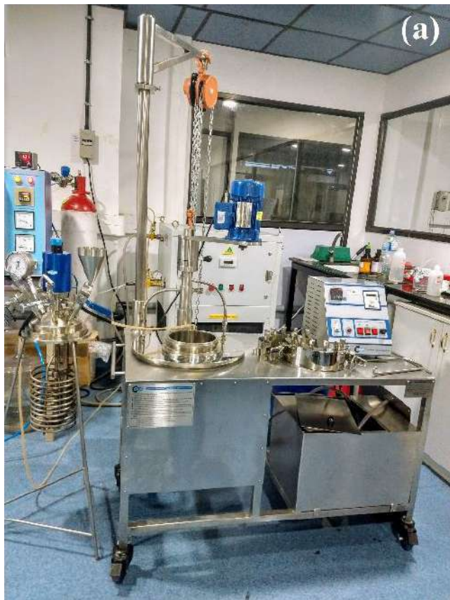
Fig.1: (a) 10L Autoclave facility and (b) sol-gel process for the scaled-up synthesis of Li-ion battery materials
